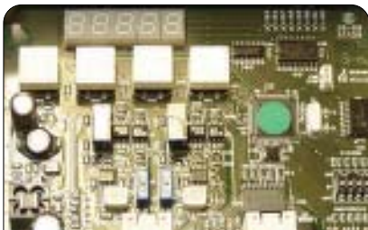
Electronic cards developed with potent micro controller and SMD technology, automatically assembled
