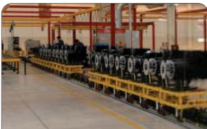
Routine testing at full load and overspeed of the totality of the alternators
